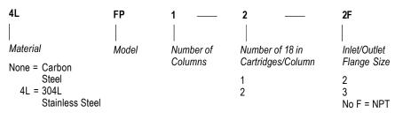
\* Operating temperature limited to 250°F (121°C) by standard Buna-N O-ring and exterior paint on carbon steel models. Optional O-ring materials are available.
